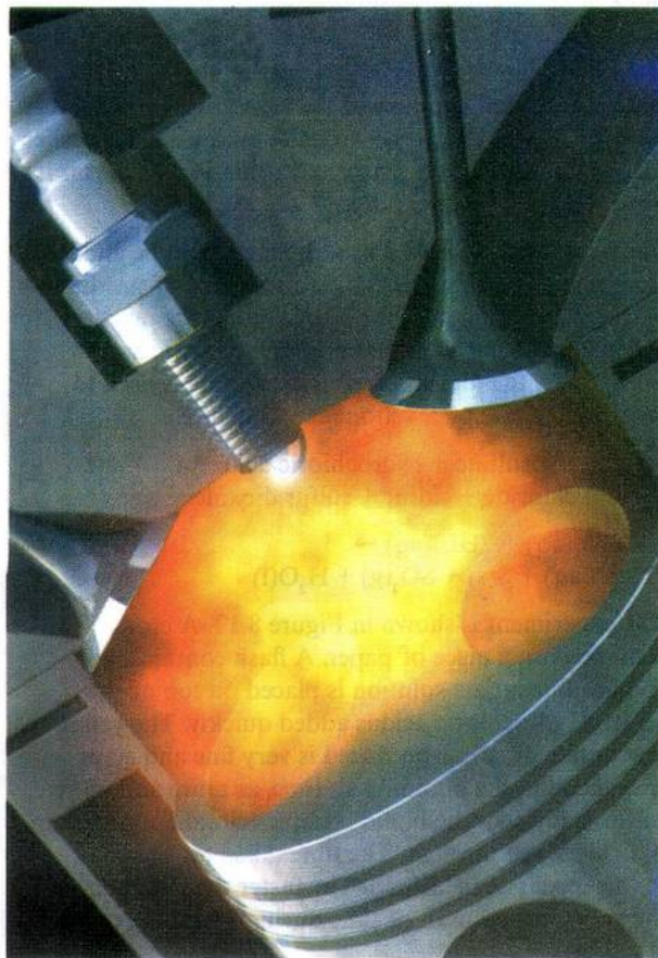
Figure 8.11: Computer graphic of the explosion within the cylinder of a petrol engine as the piston compresses the gases.
