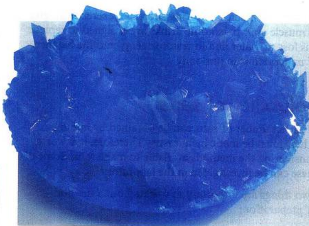
Figure 12.5: Crystals of hydrated copper(II) sulfate are blue. They contain water of crystallisation in their structure ( \text{CuSO}_4 \cdot 5\text{H}_2\text{O} ).
