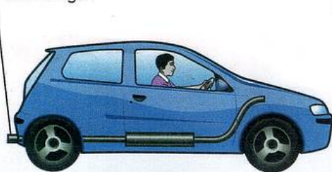
Figure 17.5: A catalytic converter converts harmful exhaust gases into safer gases.
