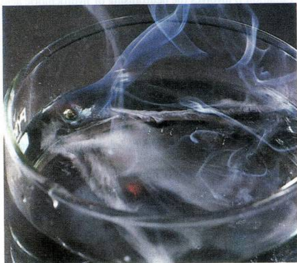
Figure 4.14: Potassium reacts strongly with water to produce hydrogen.
