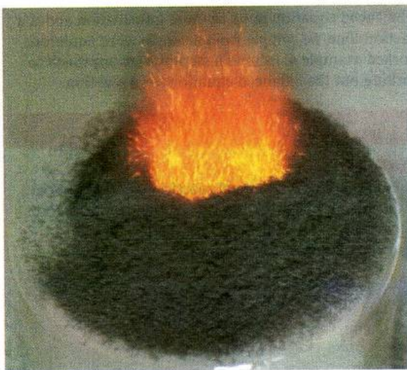
Figure 4.11: Decomposition of ammonium dichromate (the 'volcano experiment') produces heat, light and an apparently large amount of powder.
