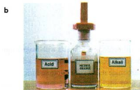
Figure 12.12 a: Colour changes for the indicators methyl orange and thymolphthalein during the titration. b: Actual colours of methyl orange in acid and alkali.
