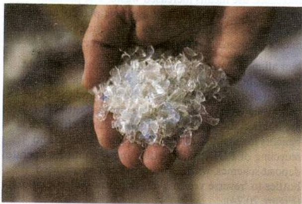
Figure 20.25: Plastic pellets (PET) produced at a recycling centre; these pellets (nurdles) will be sent for processing and reuse.
