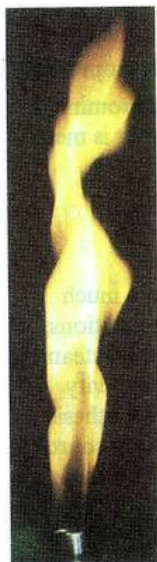
Figure 19.5: 'Safety' flame of the Bunsen burner. The air supply to the flame is restricted.
