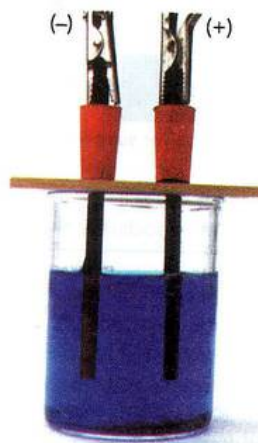
Figure 6.11: Copper is quite unreactive so it can be seen deposited on the cathode when copper(II) sulfate solution is electrolysed.
