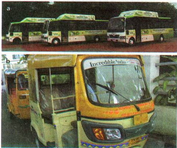
Figure 19.2 a: India's first long-range CNG buses, which can travel up to 1000 kilometres in a single fill, in New Delhi. b: A TVS autorickshaw in Chennai, India.
