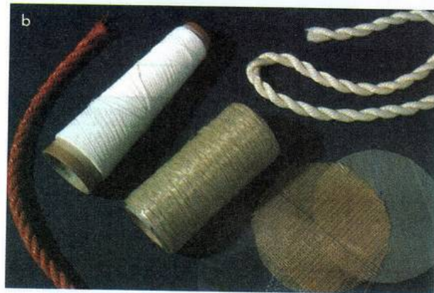
Figure 20.13 a: Plastic crates made of poly(propene) on a conveyer belt at a distribution centre. b: Different forms of poly(propene) fibres.
