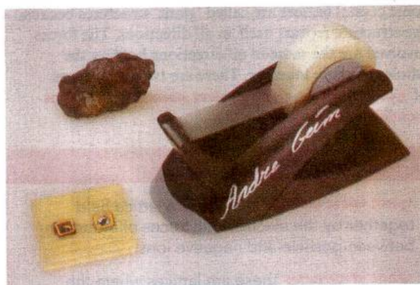
Figure 3.26: A kit for preparing graphene. Items donated to the Nobel Museum in Stockholm (a piece of graphite, a graphene transistor and a sticky tape dispenser).
