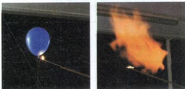
Figure 10.8 a: Balloon filled with hydrogen. b: Hydrogen reacts explosively when ignited.
