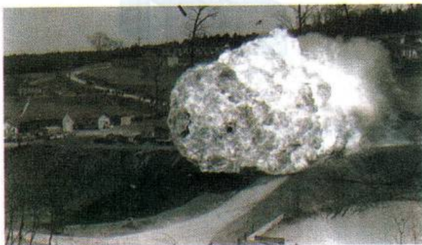
Figure 8.3: Demonstration of a coal dust explosion showing the size of the fireball that can be generated.
