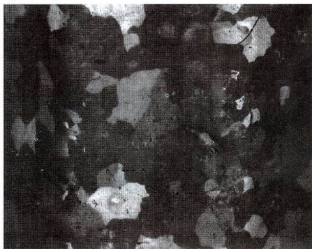
Figure 16.11: A photograph of zinc grains on a galvanised fence post.
