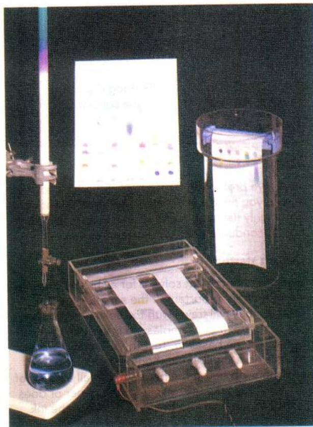
Figure 21.19: Paper chromatography is one of several different types of chromatography that work on the same principle.
