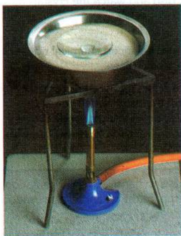
Figure 12.9: Evaporating off the water to obtain salt crystals. Here a sand tray is being used to heat the solution carefully.
