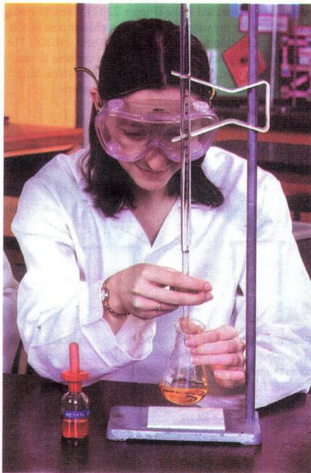
Figure 22.13: Performing an acid–base titration using methyl orange as indicator.
