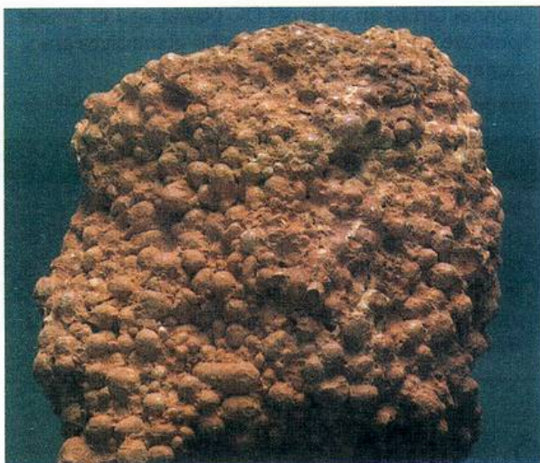
Figure 16.7: The major ore of aluminium is bauxite. Bauxite usually contains some iron(III) oxide, which gives the ore its brown colour.
