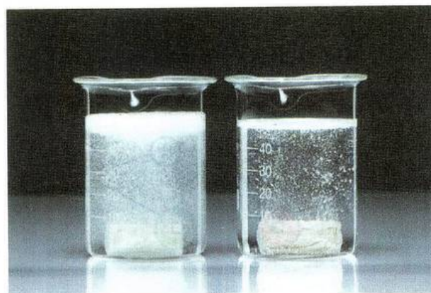
Figure 11.16: Reaction of chalk with solutions of a strong acid (hydrochloric acid) on the left and a weak acid (ethanoic acid) of the same concentration on the right.
