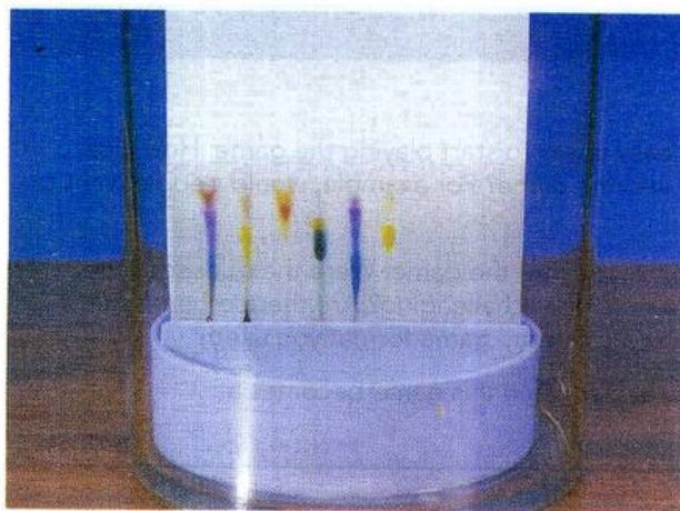
Figure 21.15: Separation of mixtures of inks by paper chromatography.
