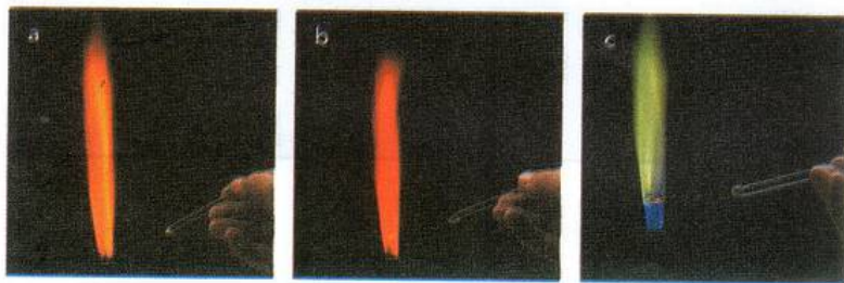
Figure 22.2: Some Group II metals give characteristic colours in the flame test: a: calcium, b: strontium and c: barium.
